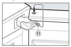
■ Remove screw ① from the hinge and screw it loosely with 3 or 4 turns into the top of the hinge pin.
